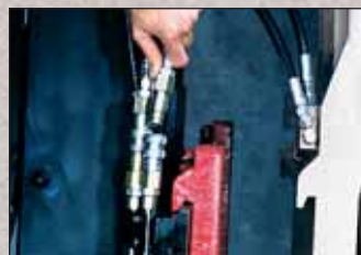
2. Connect quick change hydraulic couplers.
